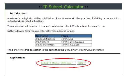
c. In the Application field, enter **192.168.50.50/27** and click **Calc!**. The next screen displays a table with network information in both decimal and binary formats.
