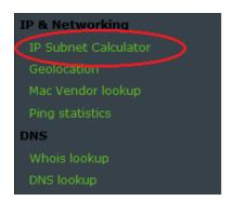
b. On the IP Subnet Calculator screen, enter an IP address and subnet mask or an IP address and CIDR prefix notation. Examples of how to enter each of these are shown in the Introduction area.
